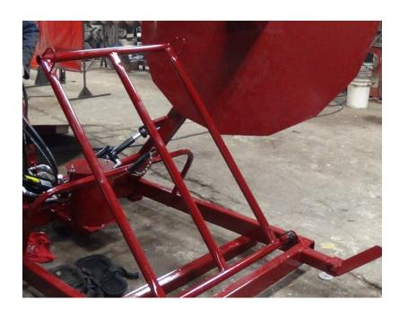
The bag tension frame acts as a bag guide and an unloading ramp.
