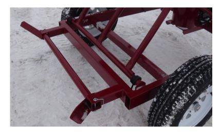
The purpose of the bag guides on the bottom of the frame are to align the bag for rolling. They also provide a vertical approach to allow foreign material to fall off.
